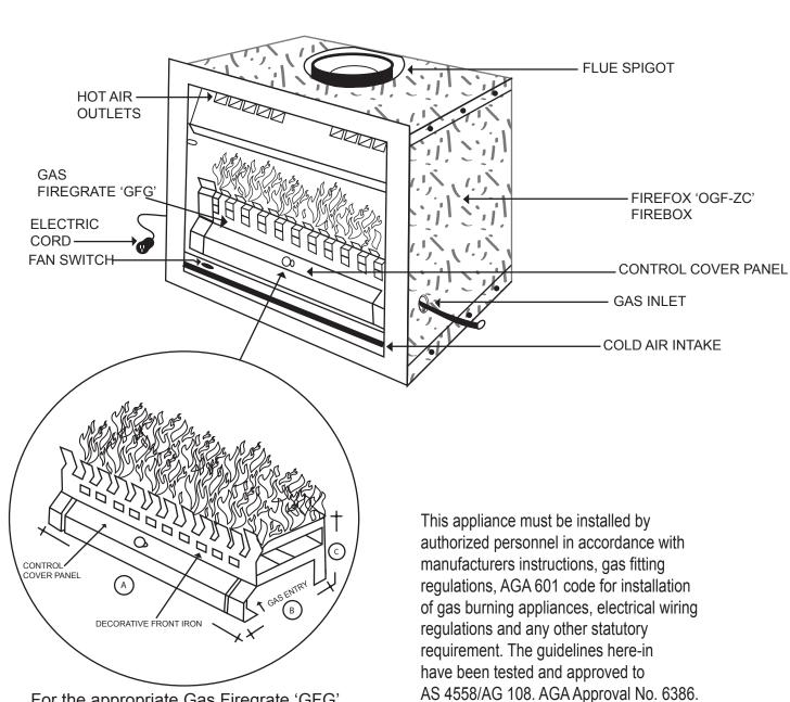
For the appropriate Gas Firegrate 'GFG' to be used in conjunction with the Gas Firebox (OGF). See specification pages on the back of booklet.
